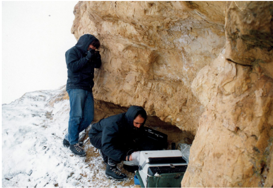
Fig. 7.14 Hiding with the noise recording equipment on a windy day with snowfall in a small cave on the lee-side of a rock cliff. Surface recordings under adverse weather conditions of the noise level at this site in NW Iran were close to the best sites in good weather.
